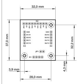
The mounting holes are 2.5mm in diameter. The solder pad holes are 0.9mm in diameter. Tolerances:
